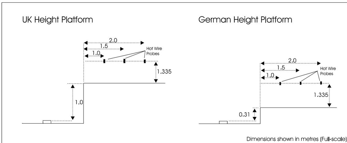
**Figure 2:** Schematic representation of hot-wire rake for passing trains slipstreams
