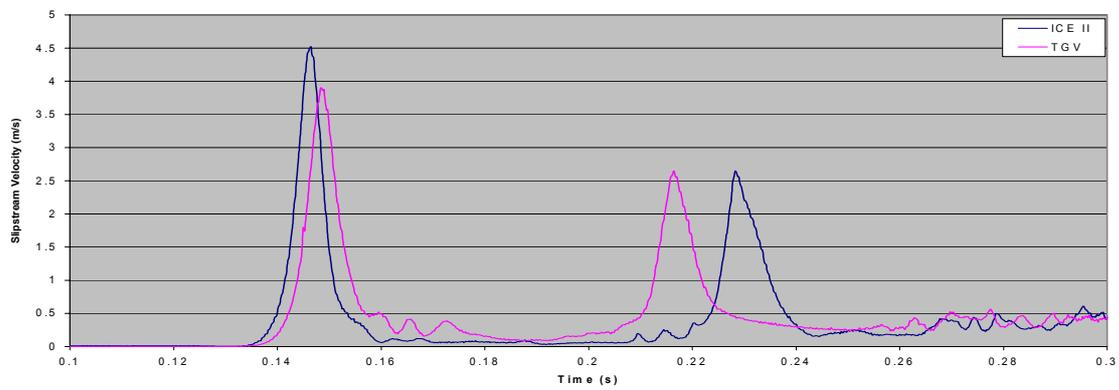
**Figure 7** *Passing Trains Runs: Mid between-tracks measurement position*
