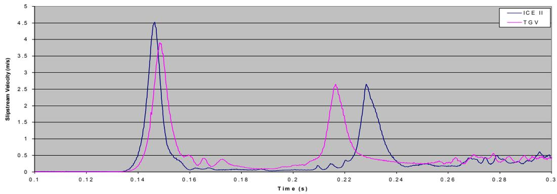
**Figure 6** Comparison of Platform Slipstream Data: Variation of Train Type
