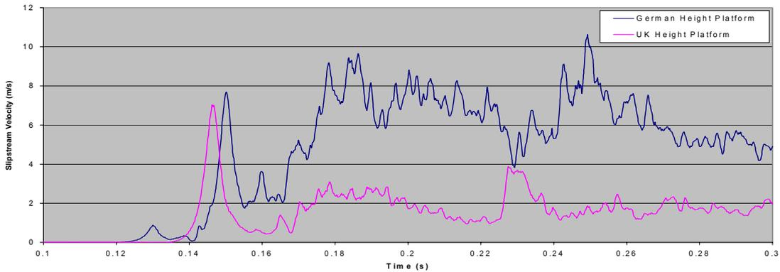
**Figure 4 Comparison of Platform Slipstream Data: Variation of Platform Height**
