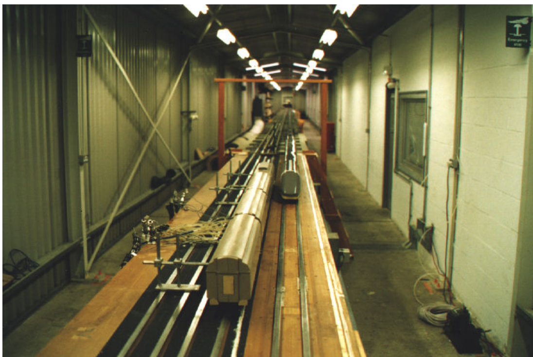
Photograph 2 ETR model (right) passing stationary freight train model (left) in the open
