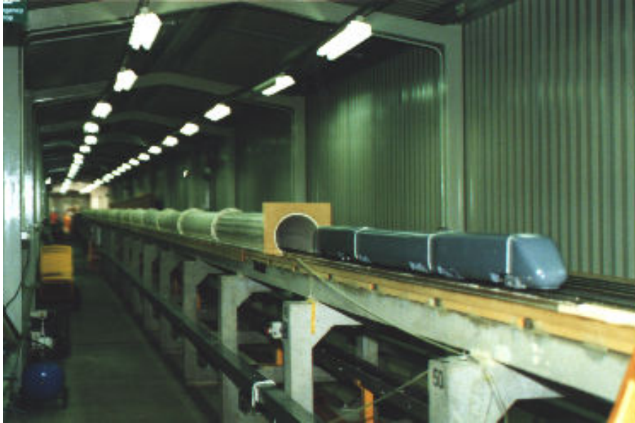
Plate 1 Porous tunnel entrance test configuration
